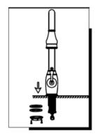
2. Install faucet through center hole assembly washer and metal washer onto faucet, and tighten with lock nut.
