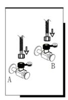
5. Attach two flexible hoses to water supply.
