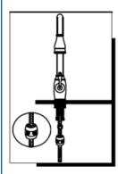
3. Proper installation of the hose weight kit will ensure that the hand sprayer retracts smoothly. On the handspray side of the hose, measure 15" down from the body of the faucet. Install the hose weight kit at this point. Pull out on the hand spray. It should move easily and retract smoothly. Reposition the hose weight kit as necessary. Make sure that the hot and cold supply hoses do not interfere with the hand spray hose. They can be repositioned slightly if necessary.
