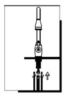
4. Screw and tighten the flexible hoses to the faucet. Do not allow the water supply brass tube to twist.
