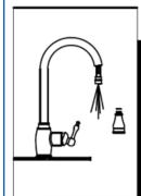
6. After installing faucet, remove shower assembly and open the hot and cold water supplies. Check for leaks. Turn on faucet handle for one minute to flush debris from faucet. Close the handles and re-assemble the shower.
