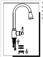
1. Remove washer, metal washer and lock nut from the faucet.
